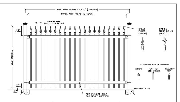
PANEL HEIGHT PANEL WIDTH POST CENTERS 101" [2565mm] UP TO 6FT, HIGH 95 ¾" [2432mm] 67 ¼" [1708mm] 7FT. AND HIGHER 72 ½" [1842mm]
